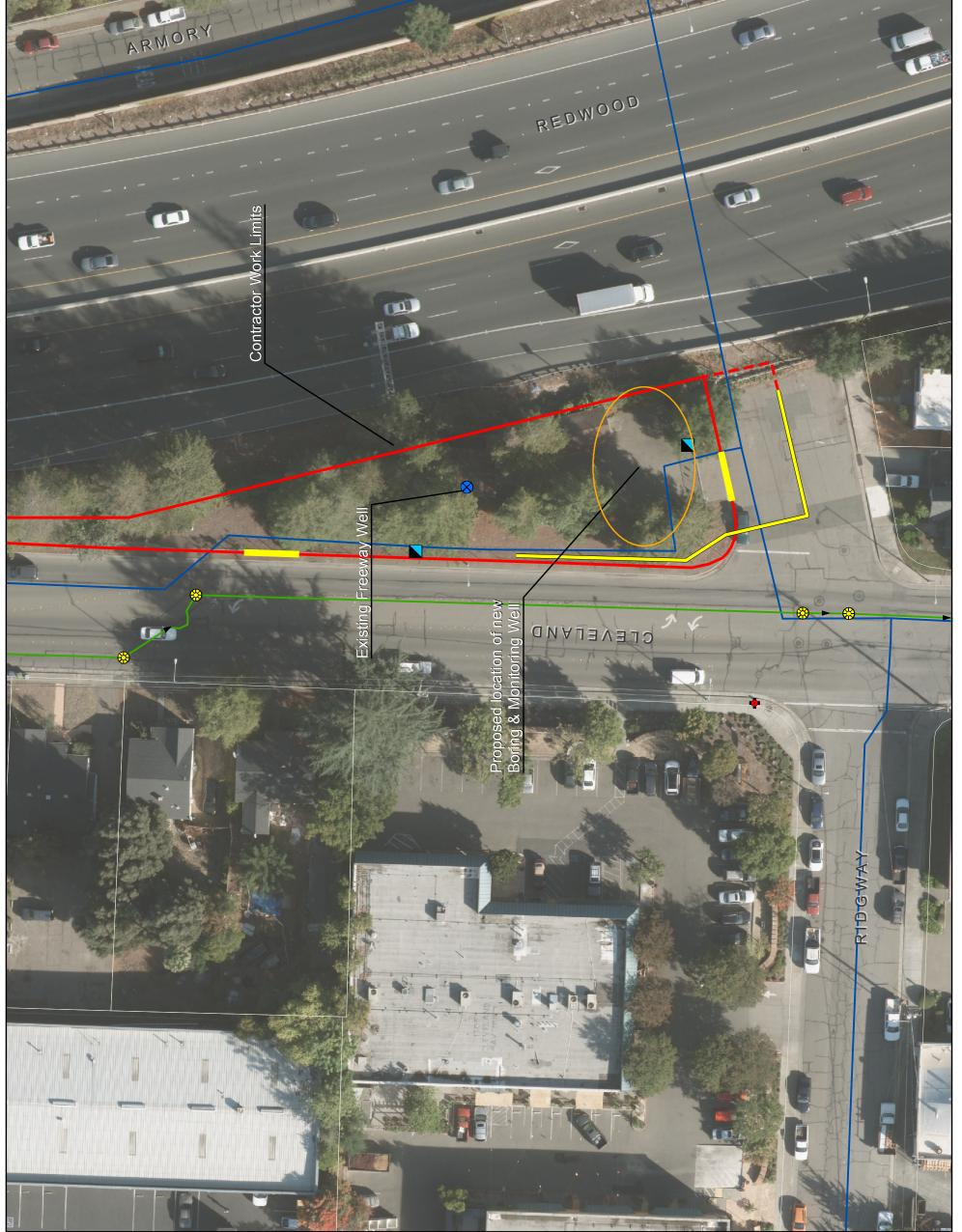
Sewer Main of 12-inch Diameter or Larger Water Source for Contractor, to be provided by City Water Main of 8-inch Diameter or Larger Temporary Construction Fence Freeway Well Site 🚯 Sewer Manhole 💠 Water Hydrant Existing Gate Soundwall Symbology Parcel I ł
